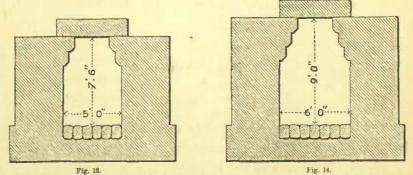
the proportions of the largest sizes built, the water-way of the one being five feet by seven feet six inches, and the clear opening of the other being six feet wide by nine feet high. These sections show the manner in which structures of this class, over three feet in width, had their walls corbelled, in order to carry the massive covering stones required.
